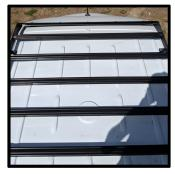
Attach your roof rack and before your 1st drive double check all fasteners to insure they are fully secured ...
