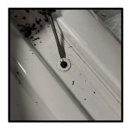
Drill out the small plastic plugs in the roof gutter in the locations that will be under the mounting feet then pop away the remaining portion with a flat head screw driver
