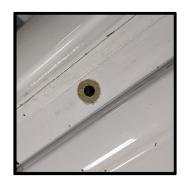
With the plugs removed you can now insert the plus nuts into the roof
