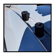
Apply more silcone to insure a water tight seal and place the spacers on the roof
