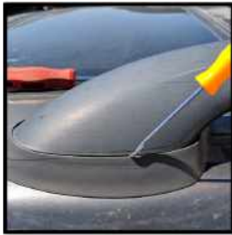
TO REMOVE THE STOCK ROOF RAILS FIRST REMOVE THE FRONT COVER BY POPPING IT UP
