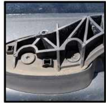
WITH THE COVERS REMOVED YOU CAN NOW ACCESS THE BOLTS TO BE REMOVED USING A T-30 BIT
