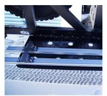
Begin by attaching the mounting feet to the crossbars. For the 5' bed you will have 4 mounting feet. For the 5.5 and 6' bed models you will have 6 mounting feet.
