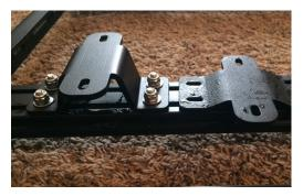
Add the washers and nylock nuts once the feet are in place and tighten them down. In some cases lower profile feet may be used.
