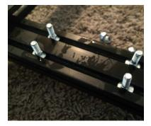
To attach the mounting feet to the crossbars first insert the carriage bolts into the tslots.
