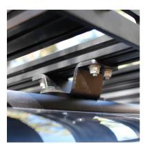
With all the crossbars install you can bolt the mounting feet into the tracks using the supplied 6mm hex bolts, lock washers, fender washers, and yakima square anchor nuts.
