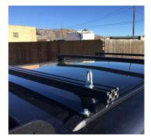
Test fit the rack by placing the mounting foot equipped crossbars on the tracks and making sure everything lines up.
