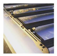
Tighten down all mounting bolts in equal increments until the entire rack is centered and secured.
