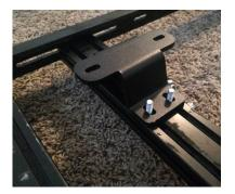
Measure the distance between the center of the tracks on your shell and place the moutning feet at that distance on the crossbars making sure everything is centered.
