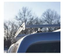
test fit the side rails to make sure everything lines up. PRINSU recommends that the bars with mounting feet be placed in the 2nd and 5th small slots on the side rails for 5' bed models. For the 6' bed models the 2nd and 6th small slots are used and then the third bar with mounting feet is placed in the middle large slot of the side rails.
