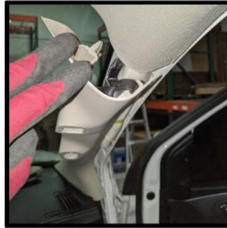
Pull away the rubber weather stripping around the door then pull back the A pillar trim
