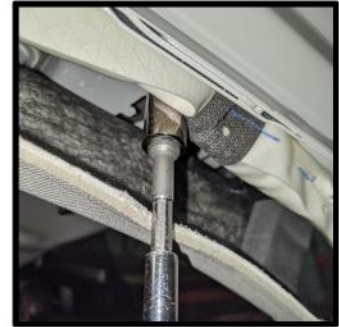
This will provide access to the bottom side of the channel trim bolt to remove the nut
