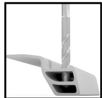
The rest of the mounting holes will require drilling thru both channel layers as shown above to a diameter of 25/64"
