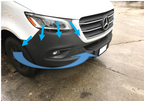
Figure 10: Removing Plastic Bumper
