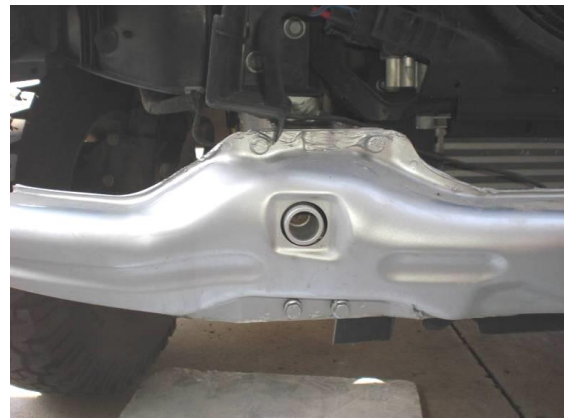
Figure 12: Four (4) of the Frame Bolts Holding the Stock Steel Bumper to the Vehicle.
