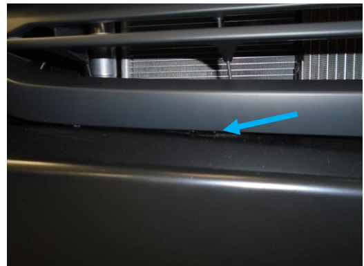
Figure 30: Grille Tabs Installed
