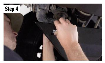
Using the longer 3/8 carriage bolt, place it into position towards the rear of the skid plate. Push it through the lower control arm and put on a washer and a nut. Hand tighten.
