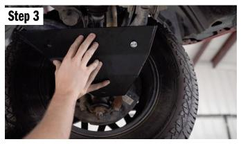
Using the shorter 3/8 carriage bolt, place it into position towards the front of the skid plate. Push it through the lower control armand put on a washer and a nut. Hand tighten.
