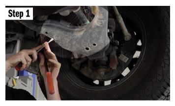
First you will need to remove the plastic caps that are located on the lower control arm. Use can use a flat screwdriver or pry bar to remove them.
