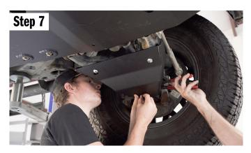
Place the remaining nut onto the 1/4" bolt, and tighten. Note: This is best installed with the vehicle on the ground. Once all the bolts are in place - tighten down all the bolts.
