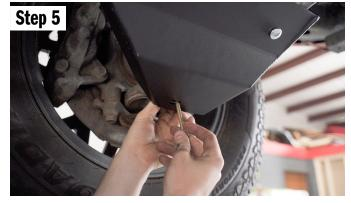
Place the aluminum spacer between the skid plate and the lower control arm.
