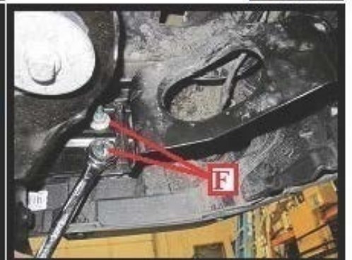
Remove 2 nuts (F) shown above both driver and passenger sides using a 16mm socket or box end wrench
