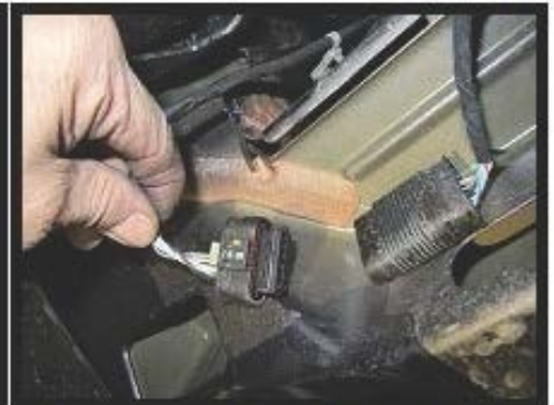
Pull out on white tab (D) in the direction of the red arrow shown in Fig. 5 to release connection lock then pull apart sensor connection (C) as shown in Fig. 6
