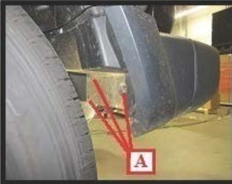
Remove passenger and driver side splash guards by removing 3 screws (A) shown above with an 8mm socket
