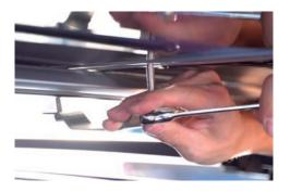
Step 8 Now it's time to orient the Roofnest so that it is centered where you want it. If the mounting hardware is loose then you should be able to move the Roofnest so that it is lined up on your roof where you want it.
