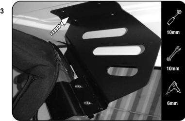
Loosely attach the Rear Support Arms (item 11) to the outside of the Roll Bar Clamps using items M6 x 20 Hex Bolts, M6 x 19 x 1SS Flat Washers and M6 Nyloc Nuts (Items 3, 7 & 8). Make sure the foot faces the inside of the vehicle and the contours of the foot match the
