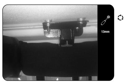
From the inside of the vehicle, in the same position as where you just inserted the bolt in Step 3.5, push the Middle Support Bracket (Item 14) through the hole in the roll bar padding and loosely fasten it to the roll bar.
