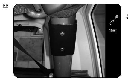
Locate the two threaded holes on the underside of the roll bar and fasten the two halves of the Roll Bar Clamps (Items ()1 & 2) to the roll bar using M6 x 19 z 1SS Flat Washers and M6 x 20 Hex Bolts (Items 3 & 8). Place the Outer Roll Bar Clamp (Item 2) first followed by the Inner Roll Bar Clamp (Item 2).
