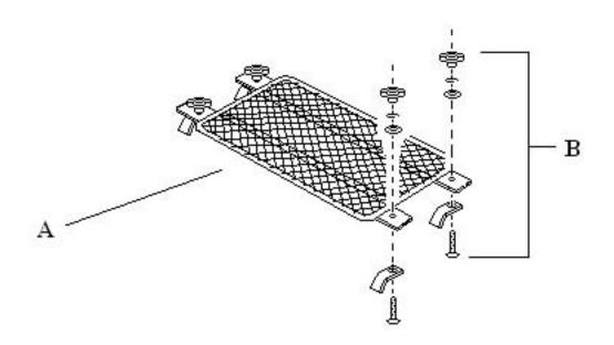
"CAUTION" When securing cargo to the H2 insert make certain that cargo straps are tied to the roof rack <u>ONLY</u> and not the H3 insert alone as this will insure the stability and security of the Gobi H2 sun roof insert and cargo from accidental movement or dislodging.
