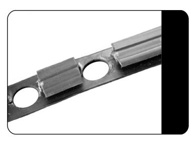
Using a 22mm hole punch (Recommended) or hole saw, punch/drill holes through the ditch molding on each of your markings.
