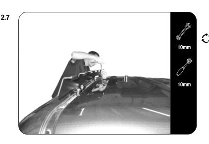
Place the side rails onto the vehicle, lining up the holes in the base of the side rails with the aluminium spacers. There is a left and a right hand side rail. The product sticker must be on the front outer side of the vehicle.
