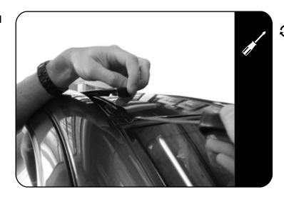
Using a flat screwdriver, starting from the front of the vehicle, lift and remove the two ditch moldings running along either side of the roof.
