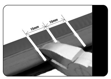
Working on the underside of the ditch molding, measure and mark a line 15mm either side of your original markings from Step 2.1 as shown in 2.2.
