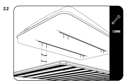
Slimeline II Rack, slide a Tent Spacer and a Tent Spacer Base (Items 3 & 4) onto the M8 x 75 Carriage Bolts.
