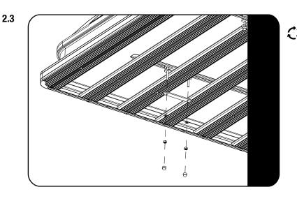
Using the remaining 4 Tent Spacer Bases (Item 3), secure the tent to the slats with M8 x 16 x 1.6SS Flat Washer and M8 Nyloc Nuts (Items 6 & 7).
