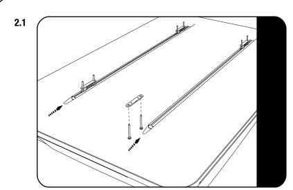
Assemble the M8 x 75 Coach Bolts and the Channel Plates (Items 1 or 2 & 5)
