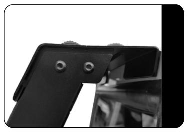
Pull the rubber door seal at the top of the inside door away from the door. Hook the top of the ladder over the top of the door. The middle lip must go between the vehicle door and the rubber door seal and the two side tabs on the outside of the door as shown.
