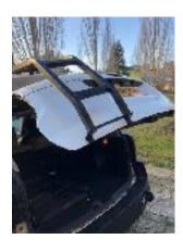
With rear door open, align bottom of the ladder parallel to the bottom of rear hatch door. Attach bottom bracket, with provided screws, to base of ladder (over the lip of the bottom door hatch), as shown in **photo 3.**
