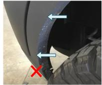
Figure 3: Fender Flare Plastic Rivets
