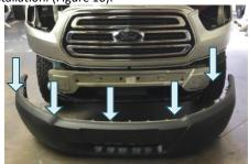
Figure 10: Front Bumper Removal
