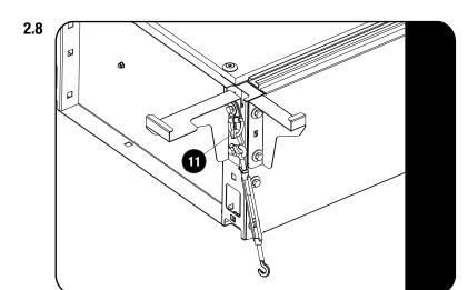
Secure the Drawer to the vehicle's front mounting points using two Turnbuckles and two 37mm Laser Cut Carabiners (Item 11) as shown.
