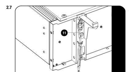
Secure the Drawer to the vehicle's rear mounting points using two Turnbuckles and two 37mm Laser Cut Carabiners (Item 11) as shown.
