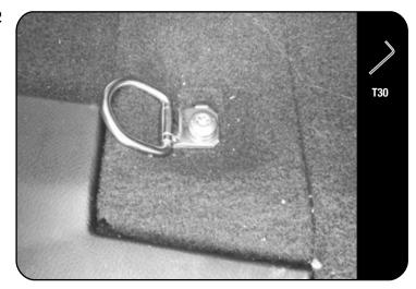
Refit the two rear tie-down points so that the D-rings face outward toward the side.
