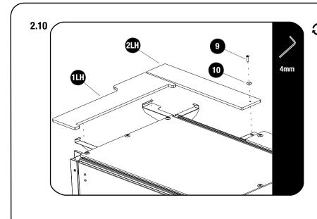
Fit the Side Decks and Rear Decks (Items 1 & 2) to the Drawer by placing them into the C-Clips and pushing downward. Secure the middle of the Rear Decks using M6 x 30 Countersink Screws and M6 Finishing Washers (Items 9 & 10) as shown.
