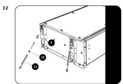
Assemble each of the 4 turnbuckles (item 12) with a wing nut (item 10) as shown. The wing nut will be used to lock the turnbuckles after they have been set.
