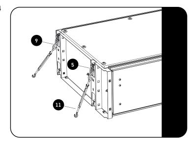
Connect the C-hooks (item 9) onto the D-rings (item 5) on the drawers upright. Connect the turnbuckles (item 11) on the other side of the C-hooks and hook it into the tie-down that are fitted to the vehicle.
