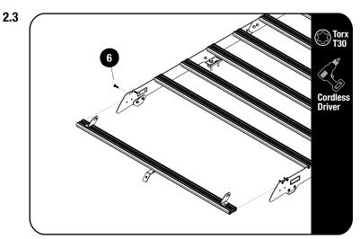
Secure assembly 2.2 to the front two top holes on the foot rails using the fasteners supplied with KSLG001.
