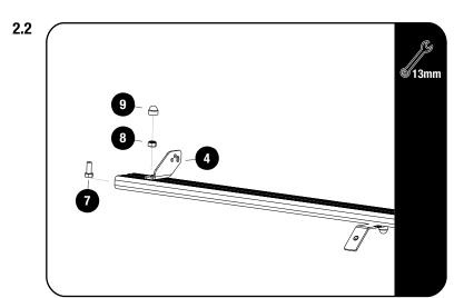
Fit the Light Bar Bracket 01 LH / RH (Item 4) for for the 40" Light Bar, using M8x16 Hex Bolt & M8 Nyloc Nut (Items 7 & 8). Fit the light bar and center it on the slat before fully tightening the brackets.
