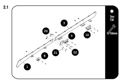
Join the Foot Rails(Item 1 & 3) together with the joiner plate (Item 5) as shown using M6x16 button head flange screws & M6 Nyloc Nuts (Items 20 & 21).
