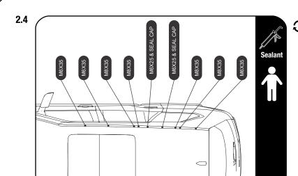
To secure the rack, the factory nuts need to be adhered to the inner roof skin. This will make the rack easily removable if needed. Unroll the 350mm long strip of VHB tape (item 29) place the eight M8 and ten M10 factory flange nuts onto the VHB tape and press down firmly (flange side down). Trim the excess tape to separate the nuts and pierce a hole with a screwdriver to allow a screw to be inserted......
