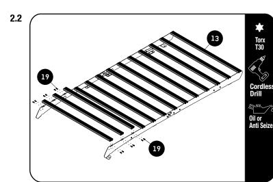
Use a little anti seize or oil on screw threads before inserting. Note these are Thread Forming Screws.
