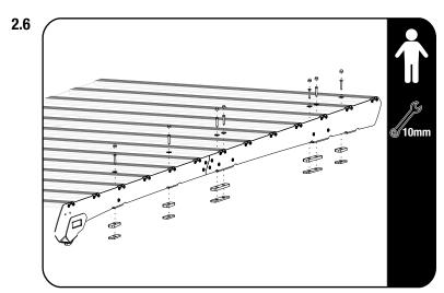
With the help of a friend lift the rack over the the roof and position it onto the spacers placed earlier.
