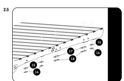
Fit the sealing cap, M6x25 Button Head Screws and M6x12x1 Flat Washers (Items 28,32 & 33) to the 4th & 5th holes from the rear. Do this on both the LH and RH side of the roof.
