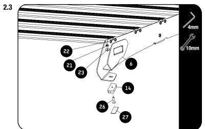
Assemble the Front wing Bracket (Item 6) to assembly 2.2.
