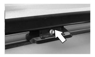
(C) Clean the area around each of the threaded mounting points and apply some silicone over each point. Place three Spacers (Item 9) over each pair of mounting points front, middle and rear as shown. The Spacers must be placed with the wider section towards the outside of the vehicle.
