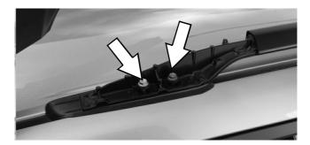
( **B** ) Remove the cover from the middle of each Roof Rail and undo the bolt as indicated by the arrow. Remove the Roof Rails from the vehicle. Remove the two remaining bolts to expose the threaded mounting points in the vehicle's roof.
