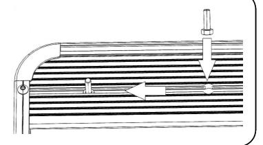
( **B** ) With your rack still upside down from Step 3A, slide a M8 x 20 Hex Bolt (Item 5) into the end of Slats 5 & 6.
