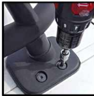
There are six torx bolts per side that will need removed
