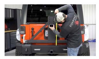
Using the tape measure, measure your wheel offset. Use this number to set the depth of the spare tire bracket. Secure the outer bracket using the remaining two (2) bolts, two (2) washers, and two (2) lock washers.
