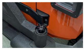
Install your tire carrier stop on the bumper using the supplied M8 hardware.
