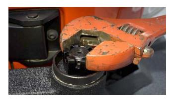
Once you are happy with the adjustments, insert and bend the cotter pin to hold the nut in position. Install the spindle cap and secure using the M6 flat head screw and a 4mm hex key.
