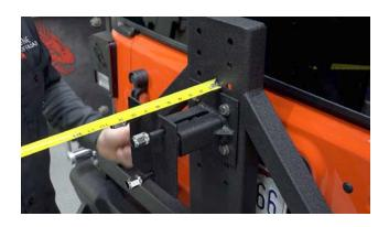
Install your spare tire using the supplied lug nuts and a 19mm socket. If all your measurements were correct, it will fit perfectly!
