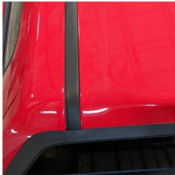
Locate the weather stripping on the top of the roof. First push up from above the rear window to begin removal
