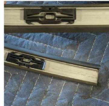
The remaining attached portion can be removed by sliding the strip backwards and then lifting up to release the clips shown above
