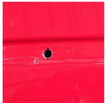
Drill one hole on both sides of the truck. The recommended hole size from plus nut is .386"-.391"*
