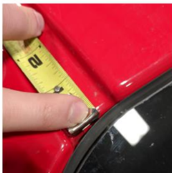
Measure from the edge of the windshield seam as shown above
