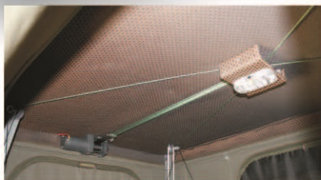
Winch and plasma rope pulley system to mechanically operate.
