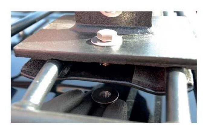
Repeat step 1 and 2 for other mounts and adjust the mounts according to your accessory, tighten the bolts with a 5/16" wrench and 5/16" ratchet tool.
