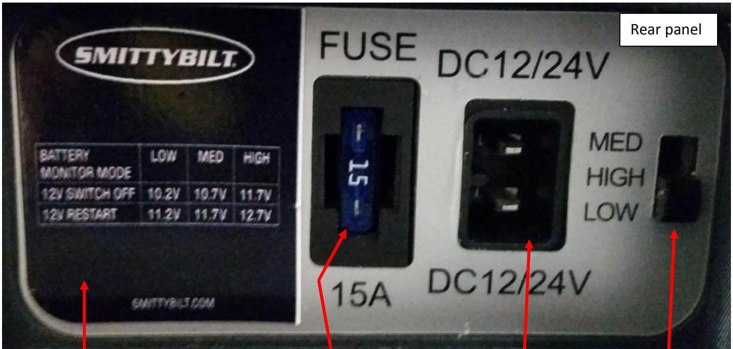
Battery monitor voltage table.
