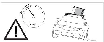
The handling characteristics of the vehicle changes when you transport a load on the roof. For safety reasons we recommend you exercise extreme care when transporting wind-resistant loads. Special consideration must be taken into account when cornering and braking.
