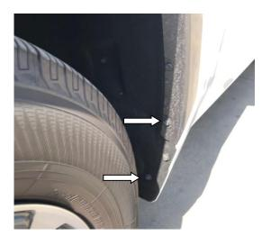
**STEP 4:** Using a 10mm socket / wrench remove the (2) screws from the inner area of the mud guard. If vehicle comes equipped with mud guard, remove all (3) screws and use a small flat screwdriver to disengage the pin from the plug at the base of the mud guard. Remove mud guards completely and retain all components. Mud Guards cannot be installed with these Fender Flares.
