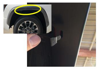
**STEP 9:** Secure attachment clips by sliding clip into Fender Flare slot and using the factory screws that were previously removed in Step: 8 to attach the clips into corresponding existing holes in upper inner splashguard. Do not fully tighten screws at this stage.
