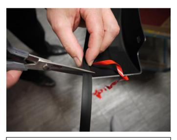
**STEP 3:** Trim rubber seal at end of each Fender Flare. Save extra rubber seal for install on opposite side Fender Flare and discard any excess once both sides are complete.
