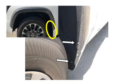
**STEP 7:** Using a 10mm socket / wrench, remove the (2) front and (2) rear screws from the inner splashguard. Retain these for later re-install.
