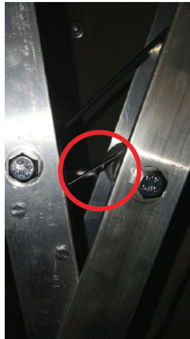
Location of Limit Switch on the arm
