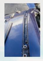
And finally on to the final installation! Lay the assembled rack on the spacers and loosely tighten the mounting bolts allowing enough room for final adjustments.
