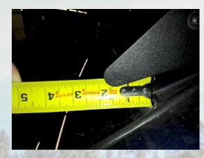
To make the install look more "factory" and help in the waterproofing, I decided to modify the rubber molding on the roof. With the rack mocked up where desired, I marked the edges of the rack mounts. Then using a Dremel, I cut out six sections of the molding where I gained access to the roof to drill for the inserts.
