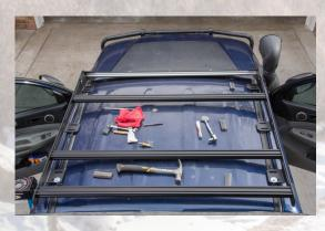
When all holes are drill and rivnuts inserted, it's time to lay down the molding and place your spacers. For the molding, I used black silicone as the sealant/adhesive, laying a bead on both sides and along the middle. Additional sealant was used around the edge of the spacers completing the seal.
