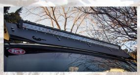
We chose to install a 40-inch Heretic light bar with our Accessrac. Prinsu offers a precut wind deflector allowing you to run a recessed light bar on the roof. So our first task was to mock up the light bar while the rack was off the truck. Prinsu provides slot nuts to run in the rails of the cross bar which is used to attach the deflector to the Accessrac.
