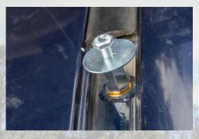
Each rivnut is designed to clamp down on the sheet metal as you tighten down with the tool. This gives you a threaded insert securely attached to your roof allowing you to now fasten the roof rack down.
