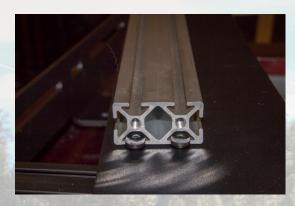
With the light bar centered on one of the crossbars, mark your mounting holes to attach the light bar.
