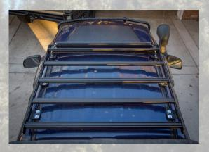
When you're happy with the alignment, tighten down all the mounting bolts (tight but not too tight), tighten down your light bar mounts as well as each cross bar and finish wiring your light bar.
