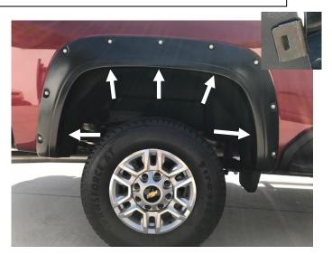
**STEP 16:** To secure the Fender Flare to the body, apply upward tension on Fender Flare to the vehicle fender when installing the black metal clips. Slide the clips over the Fender Flare and the inner wheel arch lip in the five locations shown. Position the clip so that the barb in the clip locates in the slot of the Fender Flare. Ensure all fixing points are tight and secure and that the rubber seal is flush neatly against the vehicle body. Repeat install steps for the opposite side.
