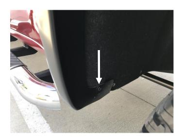
**STEP 7:** Using #15 Torx head screwdriver re-install previously removed factory mudguard screw through the slot in the Fender Flare at the noted location.
