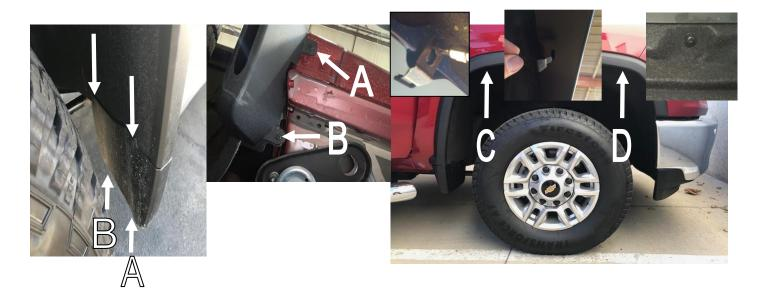
**STEP 5:** For models <u>with front</u> factory mud guards, remove factory Torx screw using #15 Torx head screwdriver at the upper x2 and lower (A and B) screw locations. Maintain #15 Torx head screws for re-install. Retain factory mudguards for later use if required, fender flares require the mud guards to be removed.
