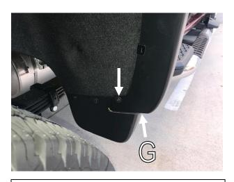
**STEP 15:** Using #15 Torx head screwdriver reinstall the previously removed factory mudguard screws at the upper and lower (G) screw locations through the slots in the front of the Fender Flare at the two noted locations.
