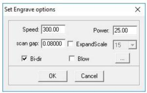
The maximum power for these machines is around 65%. The percentage controls the amount of power being sent to the laser tube and there is a peak in performance around this value. If you increase the power to 75% or 85% there is actually a decrease in cutting efficiency but you are still sending more power through the tube which will wear the tube out faster.
