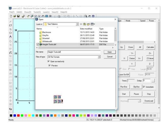
The file has to be selected by clicking on the file name, typing the name of the file into the box will not result in successful selection of the desired file.
