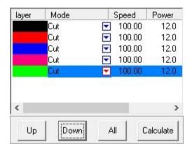
It is often beneficial to perform an engrave operation first particularly when the engraved area is also going to be outlined. The order of operations can be changed simply by selecting the desired layer and moving it up or down in the list. Select the Green layer and move it to the top, changed the mode to an engrave operation.
