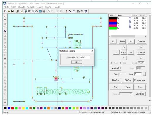
You can see that the black square on the left hand side of the drawing now has one single start point and the laser will cut the whole thing in one single motion. This function is particularly important for engraving. During the engraving operation Lasercut needs to figure out which points are inside the square so it can calculate where it needs to engrave. This is how it can tell the the letter 'o' should have a ring of black around the outside but not in the middle.
