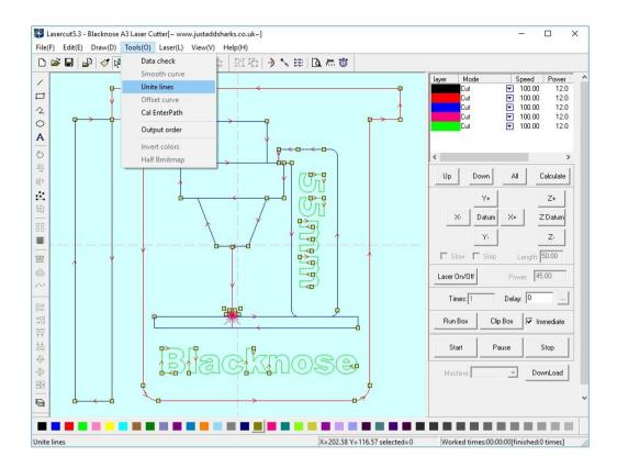
A small dialog window will open that controls how the lines are united. The dialog window asks for a value that determines how close points on the diagram should be before they are united. Enter a value of '0.01', which means if two points in the drawing are within 0.1mm of each other they will be connected into a single point. Press 'OK' to begin the merge.
