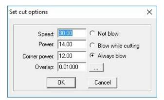
For the Blacknose laser cutter the speed should be set to 30mm/s. The Power should be set to 14% and the corner power should be 12%. This will mark the surface of the poplar ply but not cut all the way through.
