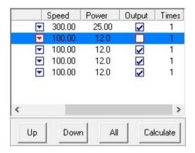
Double click the red layer to access the speed and power settings for a cut operation. This was intended to be high power and cut all the way through the material.
