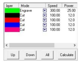
Double click the coloured section of each layer to access the speed and power settings. With the green layer set to to an engrave operation this will option the 'Set Engrave Options' dialog.
