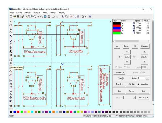
Half way down the icons on the left is a button labelled "Center to Table". Click this button to bring the item back into the middle of the work area.
