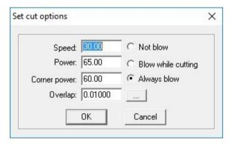
The Blacknose laser cutter is capable of travelling upto 30mm/s during a cut operation. The Power should be set to the maximum, which is around 65% as previously mentioned. The Corner Power should be 60%.
