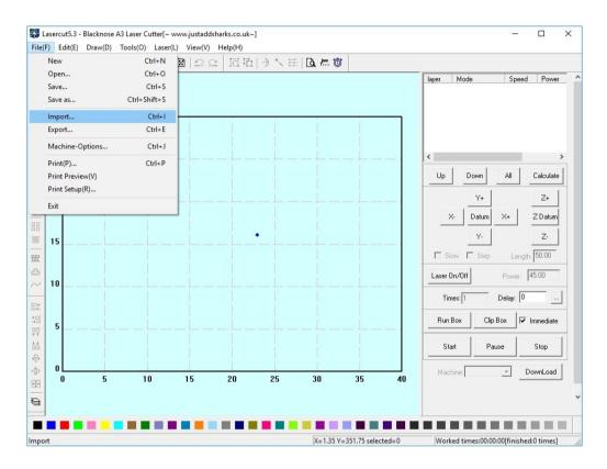
The 'Open' dialog window will appear which allows you to select a file to be imported into the program. Locate the 'Test Patterns' folder that came with the Just Add Sharks software download. Select the 'Height Tools.dxf' file and a small preview of the file will appear in the lower window once the file has been selected. If the preview does not appear the file may not import correctly. Click 'Open' once the file has been selected.
