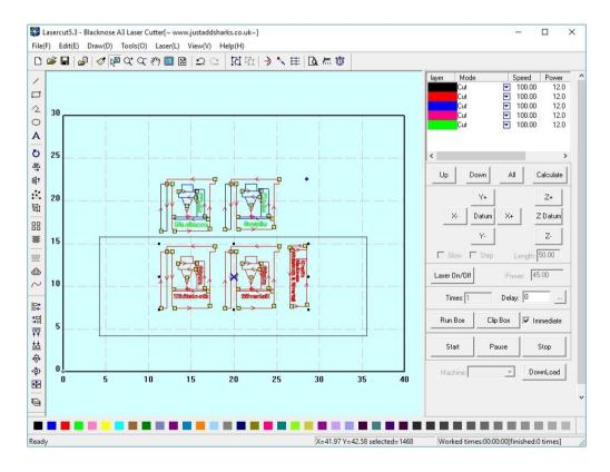
Click and drag with the mouse to select the items you don't want to cut, in the test file you should remove the height tools for the other laser cutters.
