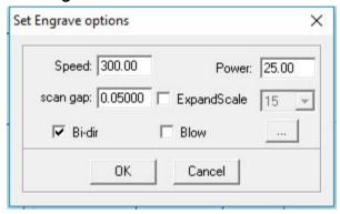
The speed is a value in mm/s that the laser head will accelerate to before engraving. The scan gap is the distance in mm, that the laser cutter will move after each row of the engraving process. It equates directly to the resolution of the image produced. The power is a value of percentage of the maximum tube power.
