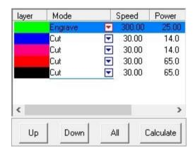
The laser will engrave the lettering first, then draw the image with low power lines and finally cut the whole thing out. It is sensible to cut the whole shape out last because once it has been cut free the shape may move around in the laser causing alignment issues between the cutting operations.
