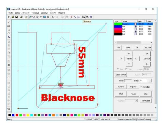
Once the artwork is prepared it can be saved in an ecp file format. This data type stores the settings for each layer so the next time it is loaded it will be ready to cut.
