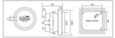
Warning: Before you connect the indicator to battery, please confirm the voltage of your battery first, and connect the positive electrode to the correct pin of the indicator on the back, wrong voltage connection maybe cause the battery indicator damage.
