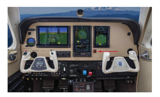
When combined with a compatible autopilot like the GFC 500/600, Smart Glide automatically activates and engages the autopilot.
