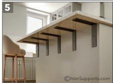
**3A. IMPORTANT NOTE:** You must make sure you are securing these brackets to a stable surface suitable for supporting the weight that will be applied. It is highly recommended that these brackets secured to a 2x4 or 2x6 stud or a header. Blocking behind cabinet carcases is a must. (see illustration for example of how to block cabinet base with a 2 x 4 or 2 x 6.)
