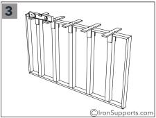
$\textbf{3} \bullet \text{ use a level to ensure the brackets are level. If necessary, use shims to } \\ \text{make the bracket level.}$
