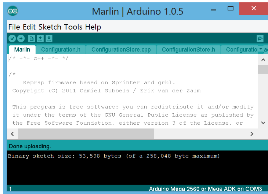
Figure 2.18: Firmware uploading done successfully
