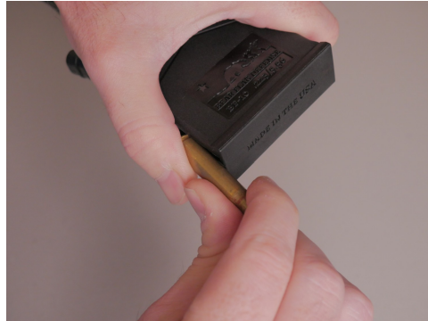
2. Use a .223 cartridge, a pen, or another similarly shaped hard object to push the cap off to the right (in the direction you read "MADE IN THE USA").
