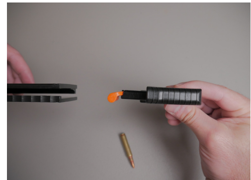
6. To reassemble, ensure follower is installed correctly as shown.
