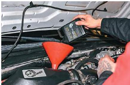
The additive will raise the TBN (total base number) of the oil it is added to, allowing oil to last longer before becoming acidic and needing to be replaced. AR9100's esters resist oxidation, further stabilizing host oil and reducing deposit formation. This extends oil life dramatically, saving money and time.
