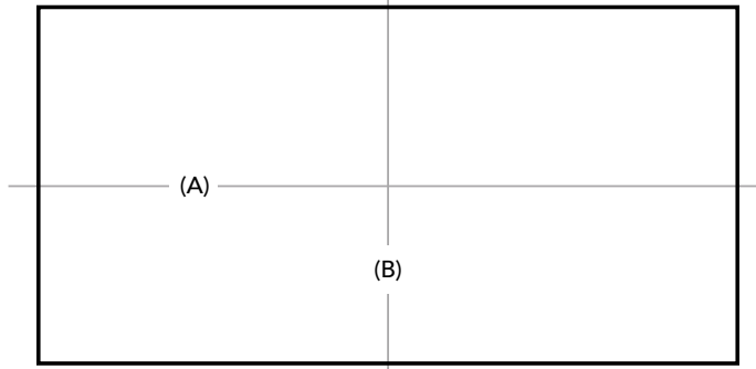
FIGURE 26 Horizontal and vertical lines for tile layout
