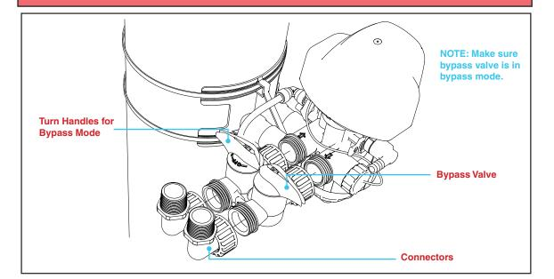
Turn off main water supply and open nearest cold faucet to relieve pressure. Cut water supply line, and connect plumbing to the inlet and outlet accordingly. Note: Inlet and outlet connections are 1" NPT. Additional piping and / or fittings may be necessary
