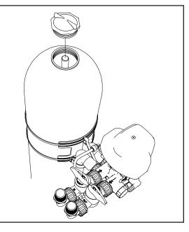
After media is added, remove the plug from the distributor tube, and fill the tank the rest of the way (up to the bottom of the tank threads) with water. This will allow the filter media to soak while the installation process is completed. Make sure that tank threads are clean and free of any media fines, and screw the control valve back onto the tank.
