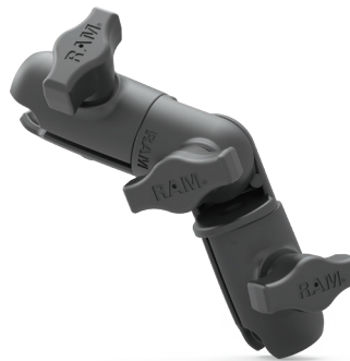
RAM-B-200-2 Overall length: 6.25" Socket-to-socket: 5.625"
