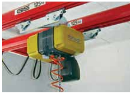
DOUBLE BRIDGE SUSPENDED CRANE
