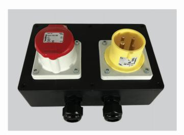
To Compliment our range of guardian controllers, the intermediate connection box enables a fixed local plug in point for chain hoists for installation applications. The Control box comes in a robust enclosure with glands included for securing of cable into the box and Din Rail terminals for easy and quick connection to the ceeform connectors.
