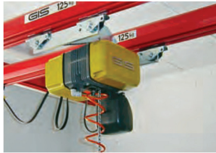
DOUBLE BRIDGE SUSPENDED CRANE
