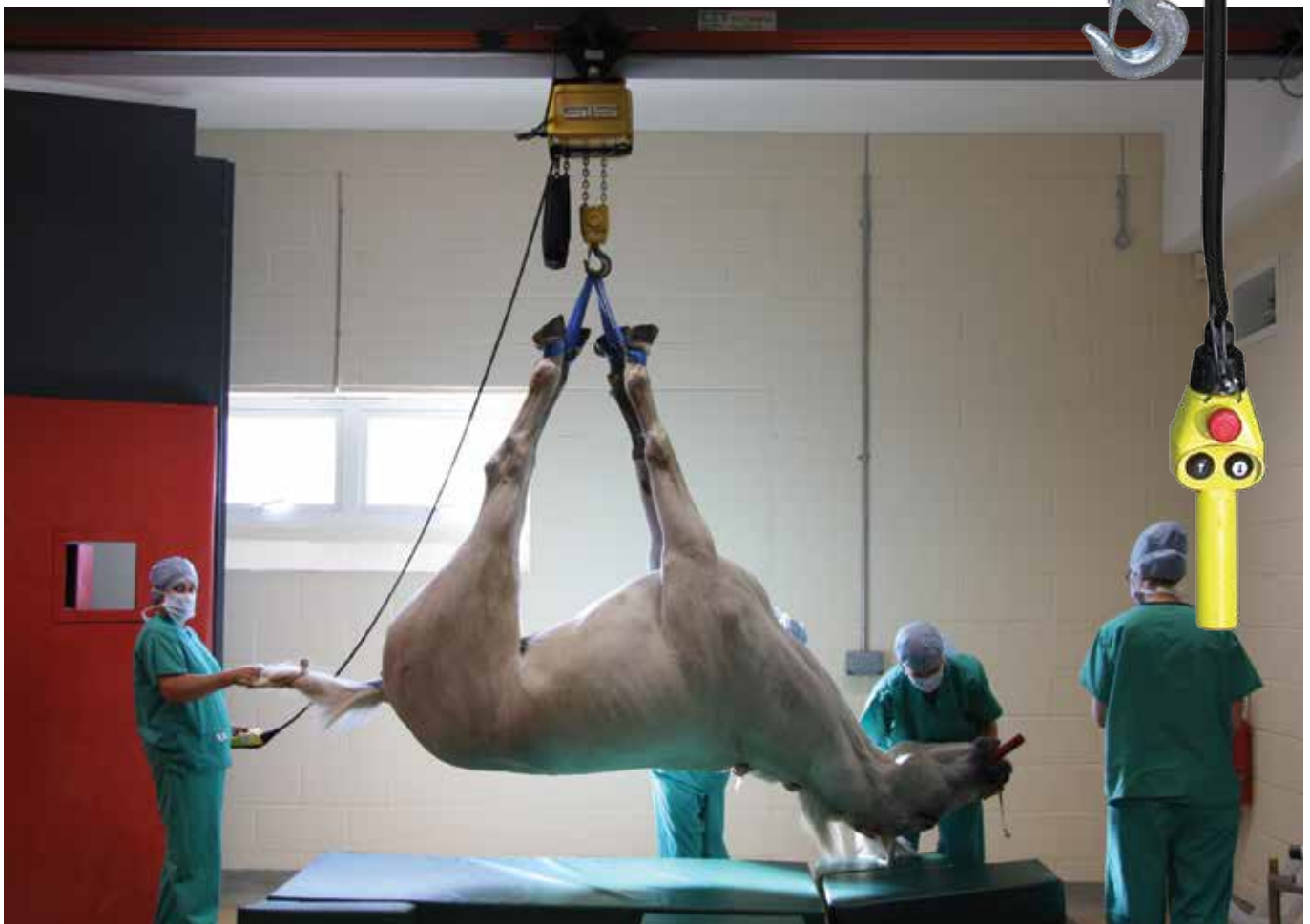
GIS HOIST USED IN AN EQUINE VETERINARY TO TRANSPORT HORSES FOR SURGERY
