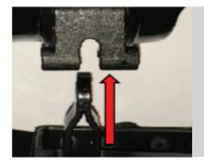
Slip the chainstore as shown in the slot of the load chain holder
