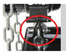
Fix the loadchain of the hoist with a screw with locknut M6x30 in the hole of the chainstore
