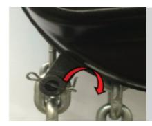
Straighten the splint and remove it from the load chain holder
