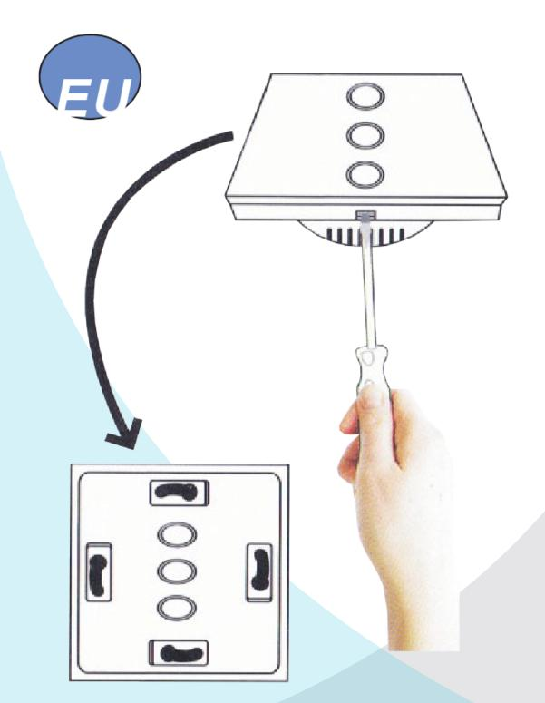
(Noted: Install without electricity power on)
