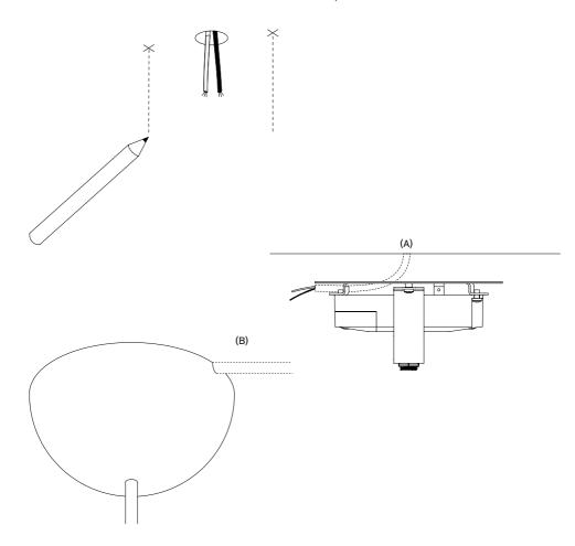
Drill holes and insert wall plugs. Ensure you use the correct type of drill and anchor for the type of ceiling you are drilling into.
