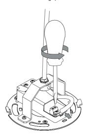
Use a pencil to mark fixing holes in the ceiling where the pendant is to be mounted. If there is a junction box in the ceiling, then the steel bracket has slots which can be used in conjunction with standard European and US junction boxes. If relevant, the input mains cable can be inserted through the centre hole in the steel bracket and passed beneath the LED driver. The input mains cable can also be inserted through the mousehole
