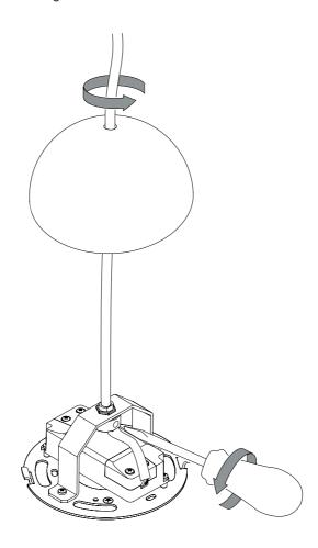
Loosen the two screws holding the terminal cover and remove the terminal cover.
