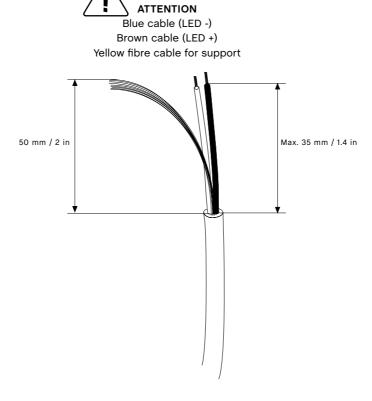
It is advised that any wire exposed with just a single basic layer of insulation is covered with the protective heat shrink provided. (Two sleeves for the basic insulated wire and one sleeve for covering the opening of the source cable). A heat gun can be used to shrink and fix this protective insulation in place (2). The double insulated mains power cable that connects to the LED driver should have a diameter between 2 x 0.75 mm<sup>2</sup> - 2 x 1.5 mm<sup>2</sup>.
