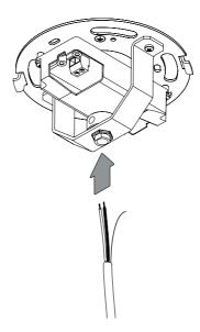
After inserting the cable through the cable grip, as shown in the previous step, locate the fibre support cable and feed it through the small hole next to the exit hole on the cable grip (1). Once the fibre support cable has exited the other side, as shown below, the smaller fixed screw on the side of the cable grip can be fastened with the provided hex key, securing the fibre support cable in place (2).
