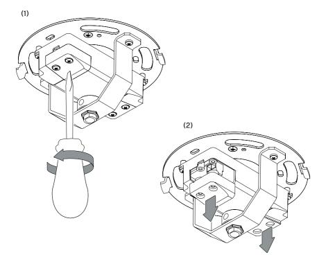
Loosen the screws on the terminal blocks so that the cable can be inserted when wiring.
