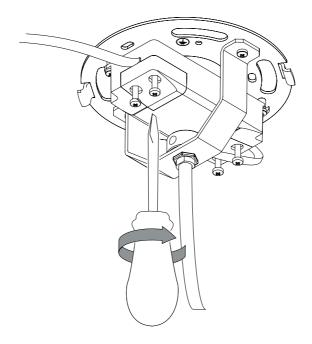
Adjust the cable from the light source, making sure that it is not pulling on the LED driver or in way of the plastic canopy. Tighten the cable grip again and make sure that the cable cannot be moved. The plastic canopy can now be replaced on the bracket.
